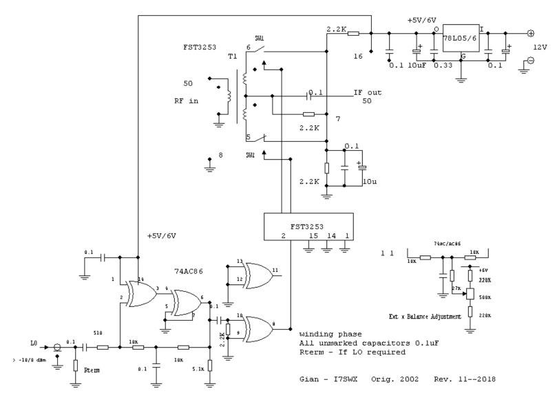
T1-T2 Prim 4 Turns, Sec 4 Turns bifilar on balun core #43-2402
