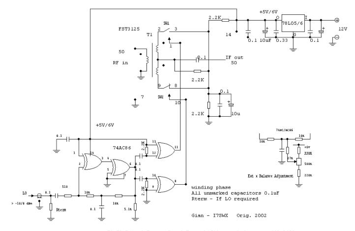
T1-T2 Prim 4 Turns, Sec 4 Turns bifilar on balun core #43-2402
