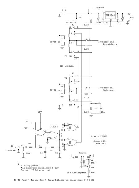
The simple I7SWX 1T Mixer using FST3125 and squarer 74AC86 as a splitted demodulator and modulator for a simple HF transceiver.
