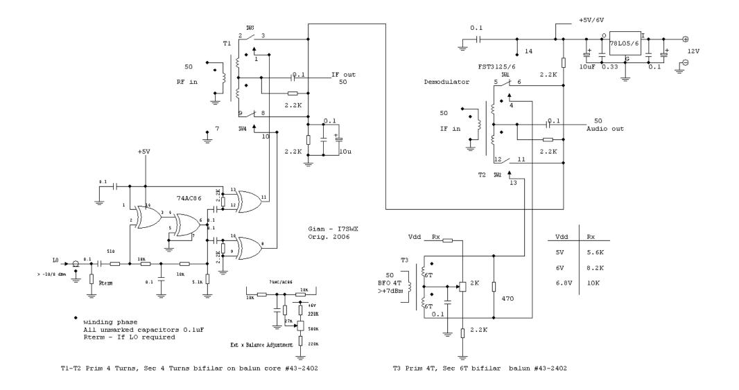
This is an example of how the simple I7SWX 1T Mixer can be utilized as an HF Front end conversion, using a 74AC86, a balance adjustment can be applied between pins 2 and 6. A simplified 1T demodulator is suggested with direct LO driving.
