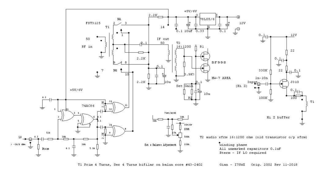
This schematic is a suggested mod for replacement of the Heath Kit HW7 mixer with the I7SWX 1T Mixer.
